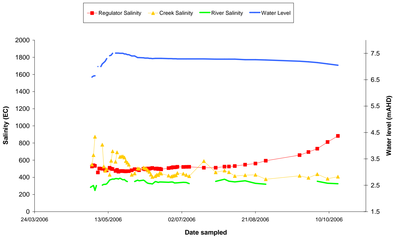
Figure 6. Wetland salinity levels (EC in \mu\text{S}/\text{cm} ) during the pumping projects undertaken in a) 2004 and b) 2006. [Source: Overland Corner Wetland Group]
